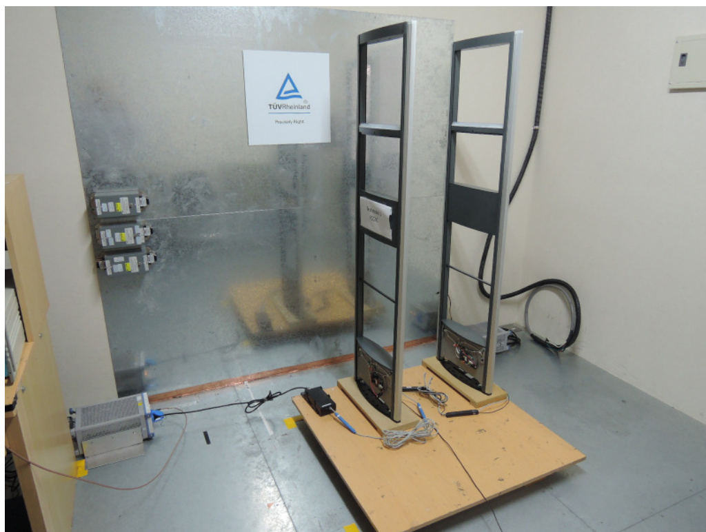
Photograph 5: Set-up for for Mains Conducted testing Front
