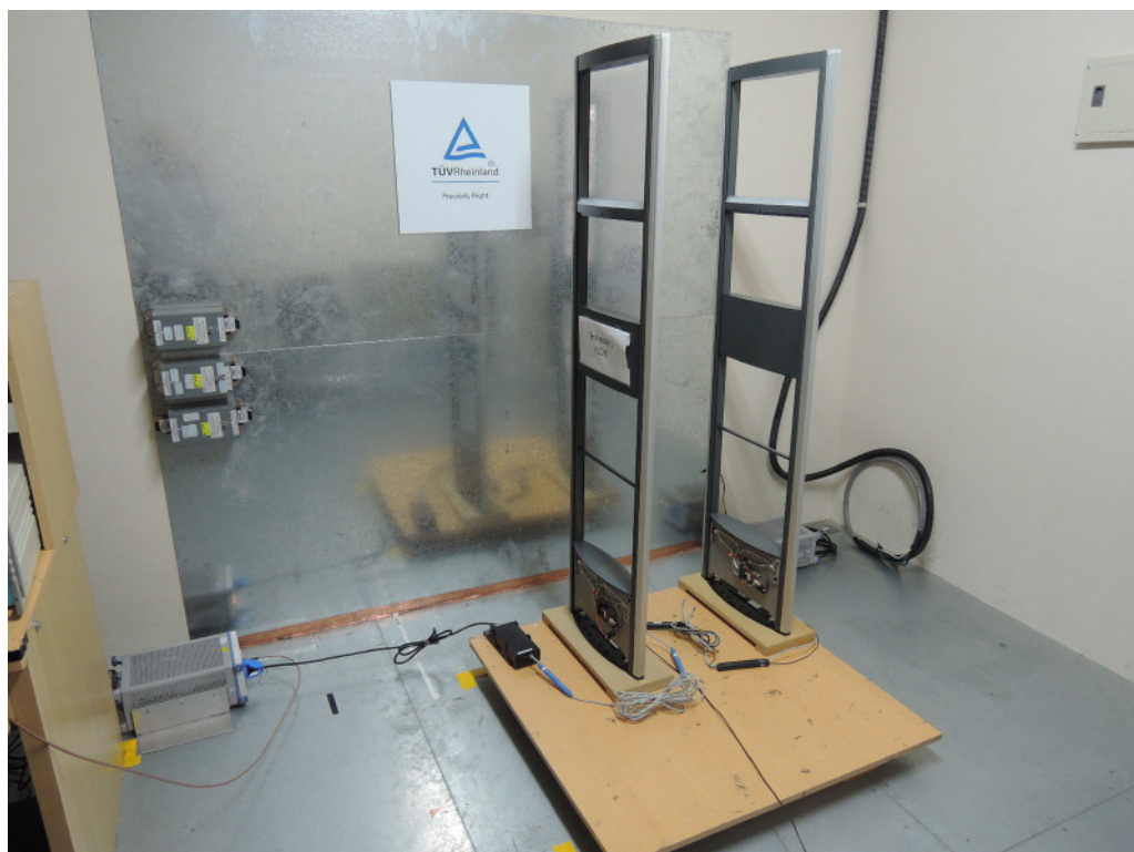
Photograph 5: Set-up for for Mains Conducted testing Front
