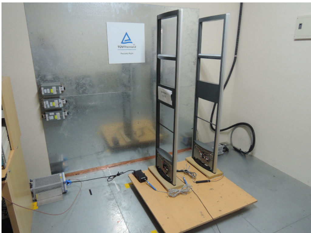
Photograph 5: Set-up for for Mains Conducted testing Front
