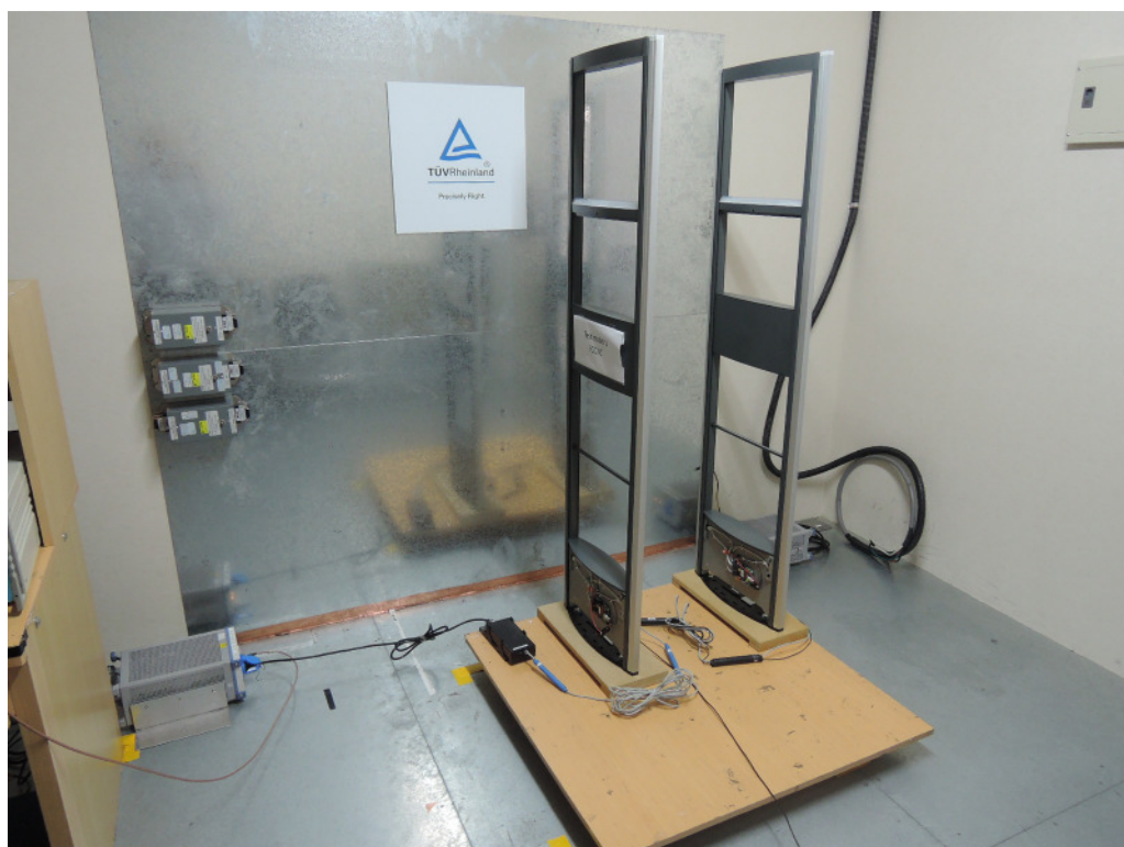
Photograph 5: Set-up for for Mains Conducted testing Front
