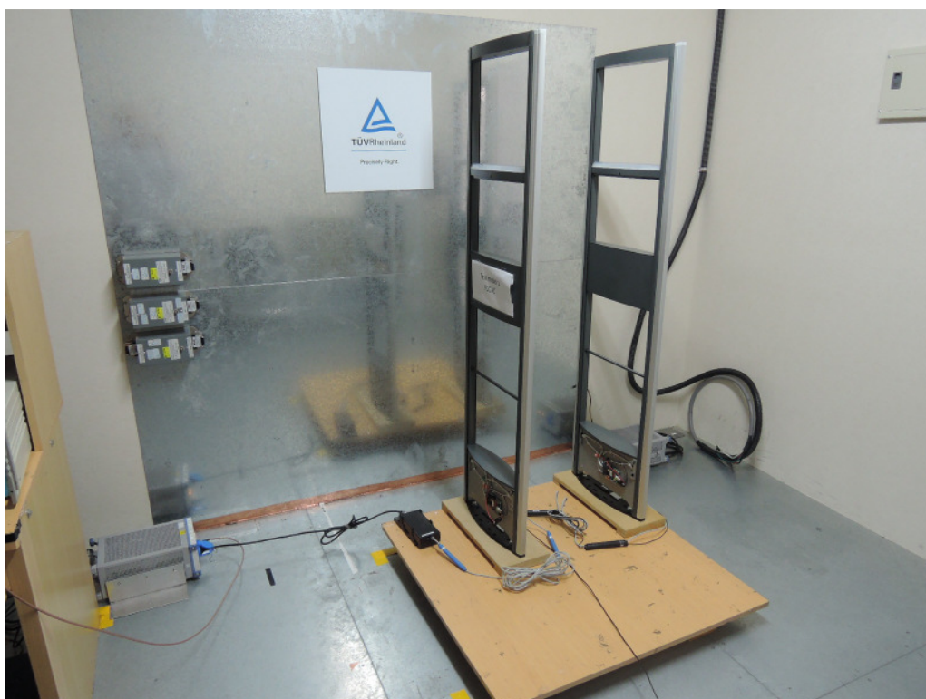
Photograph 5: Set-up for for Mains Conducted testing Front
