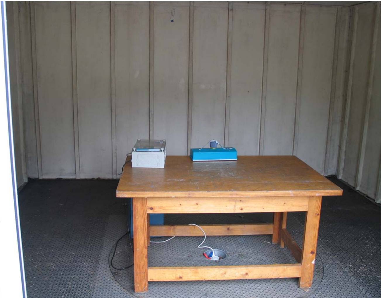
Photo 9: Radiated Emission measurement set up, front view, with AE-6 (responder) in field.
