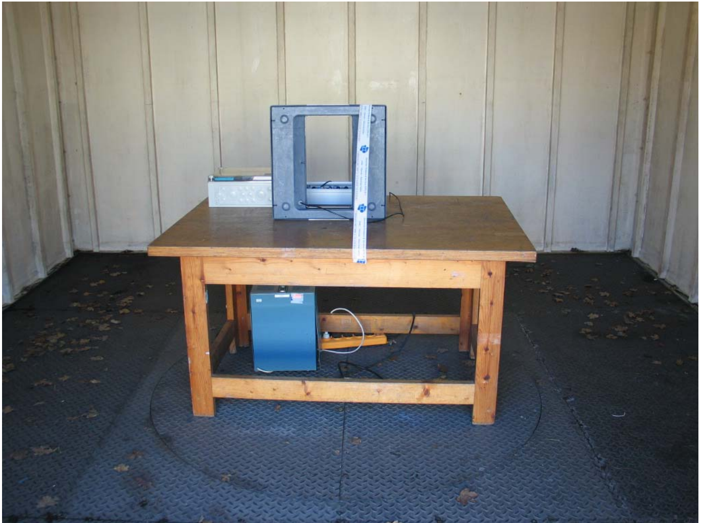
Photo 5: Radiated Emission measurement set up, front view, with medium V-sense
