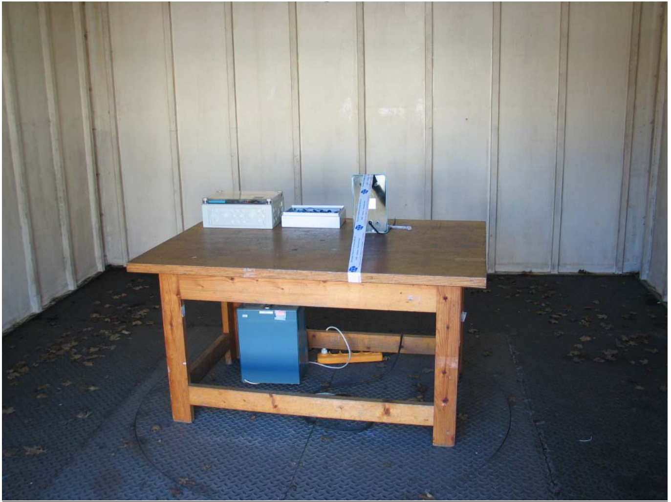
Photo 2: Radiated Emission measurement set up, front view, with small V-sense
