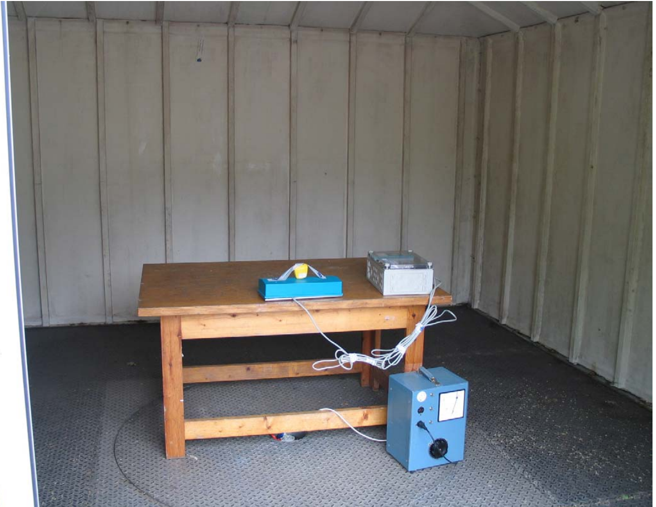
Photo 8: Radiated Emission measurement set up, front view, with AE-6 (responder) in field.
