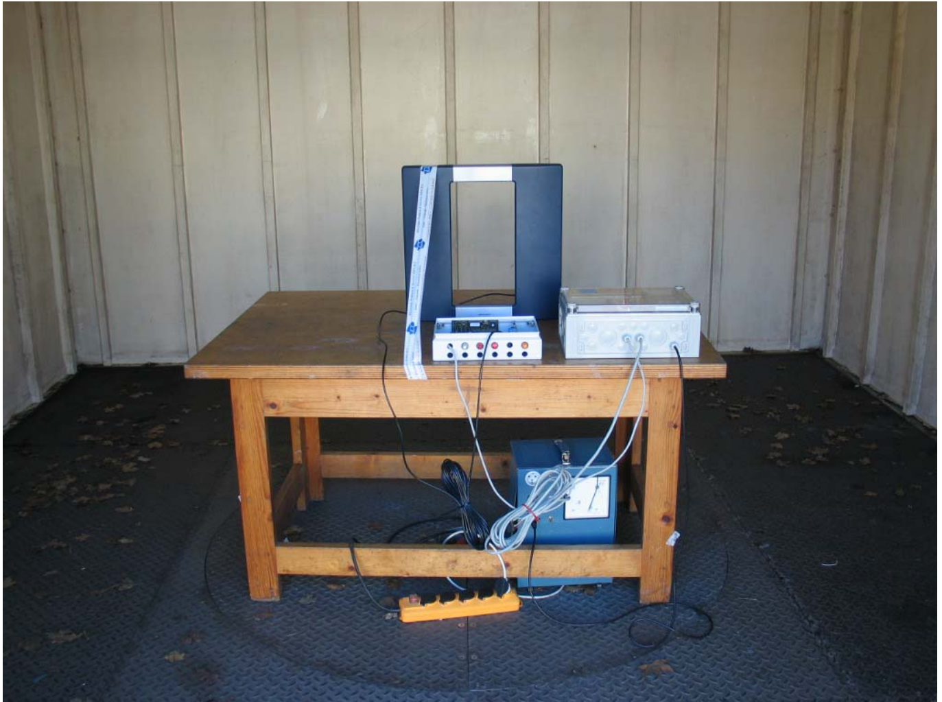
Photo 4: Radiated Emission measurement set up, rear view, with medium V-sense
