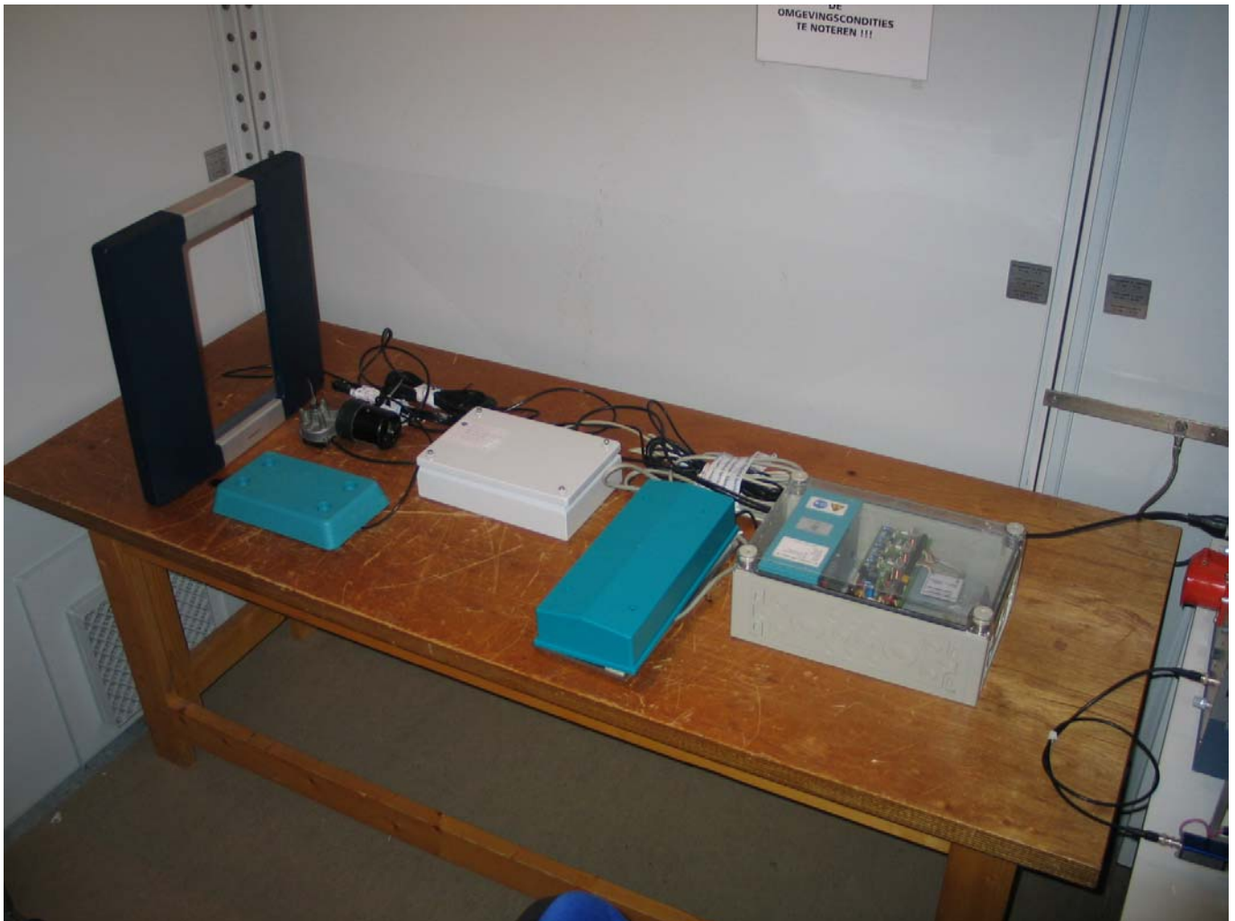
Photo 10: Conducted Emission measurement set up
