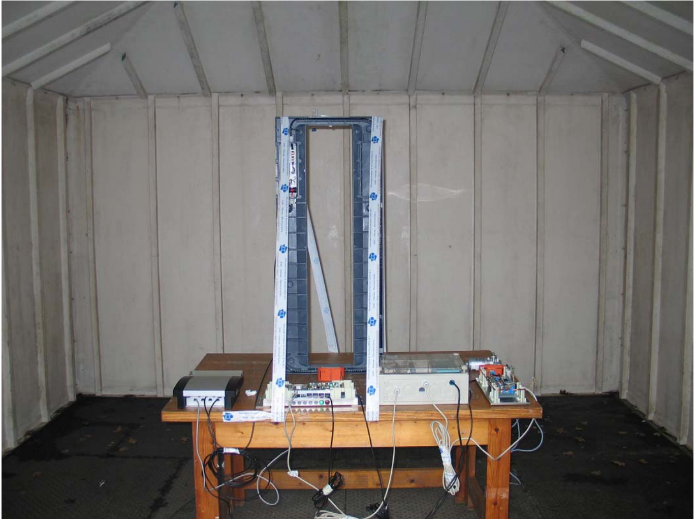
Photo 1: Radiated Emission measurement set up, rear view, full configuration.
