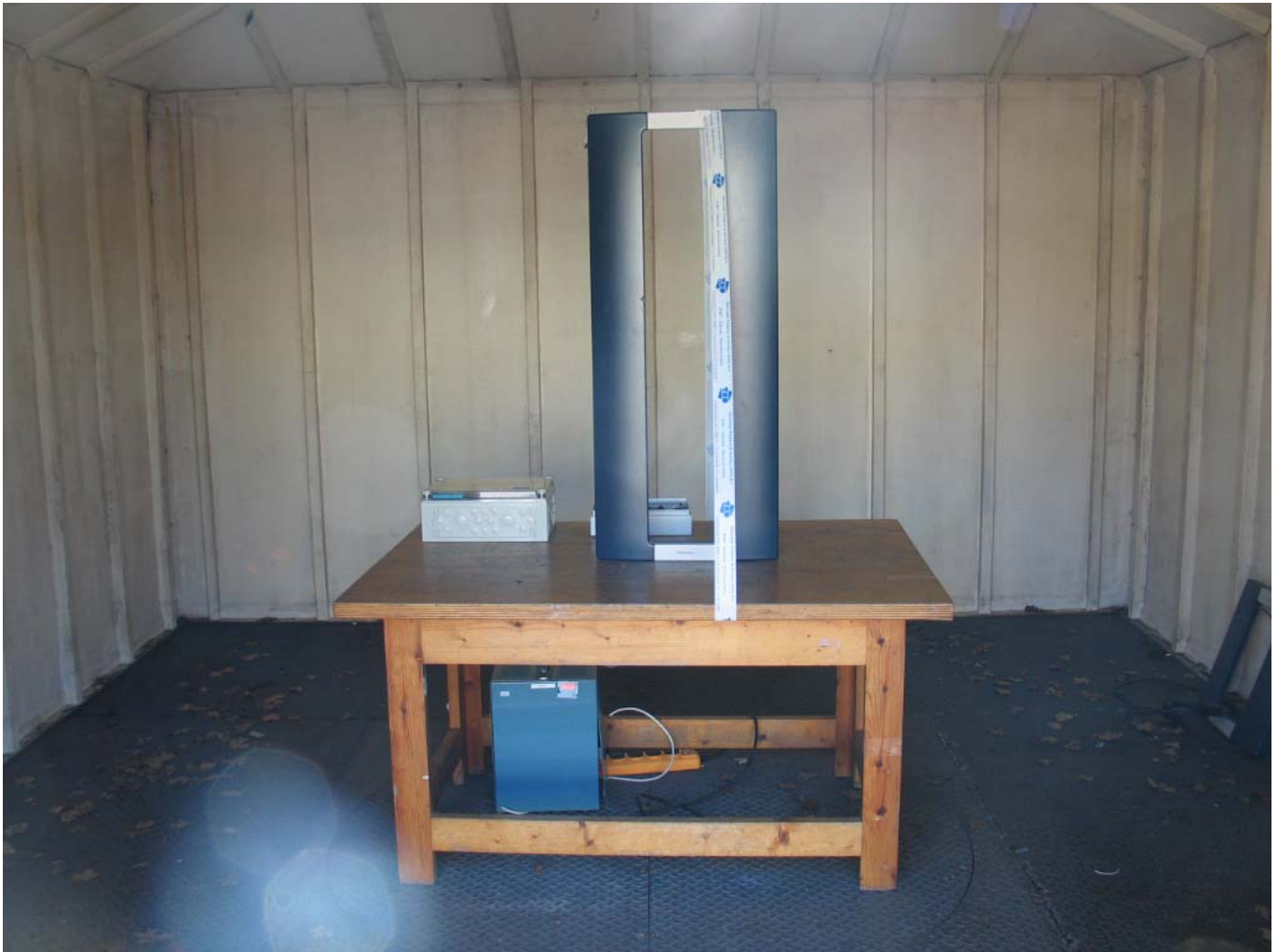
Photo 6: Radiated Emission measurement set up, front view, with large V-sense
