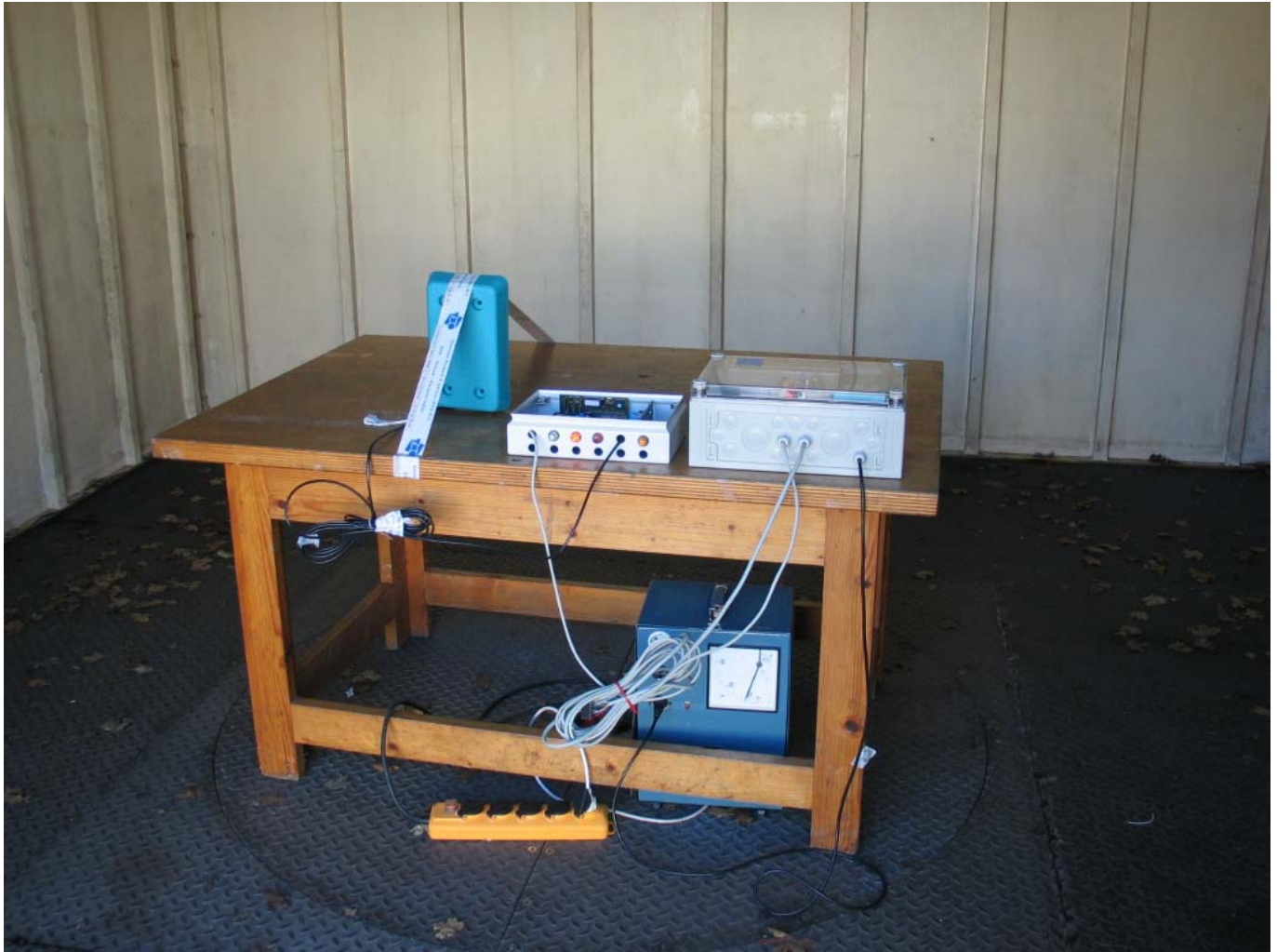
Photo 3: Radiated Emission measurement set up, front view, with small V-sense, rear view
