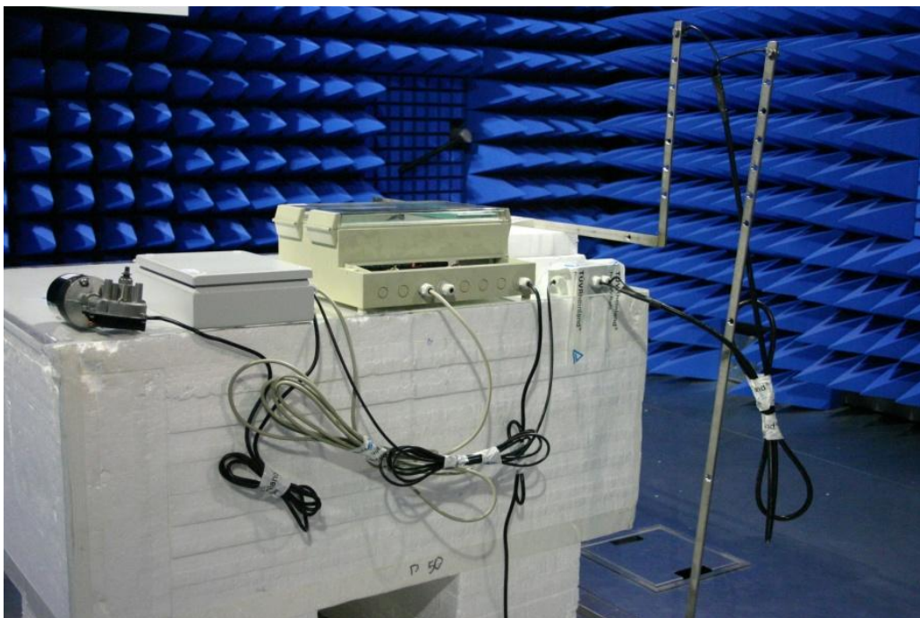
Setup showing EUT in combination with Single Loop Over Trough antenna
