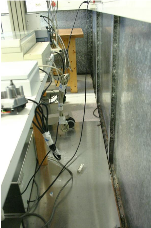
Photo . Detail test set-up conducted emission
