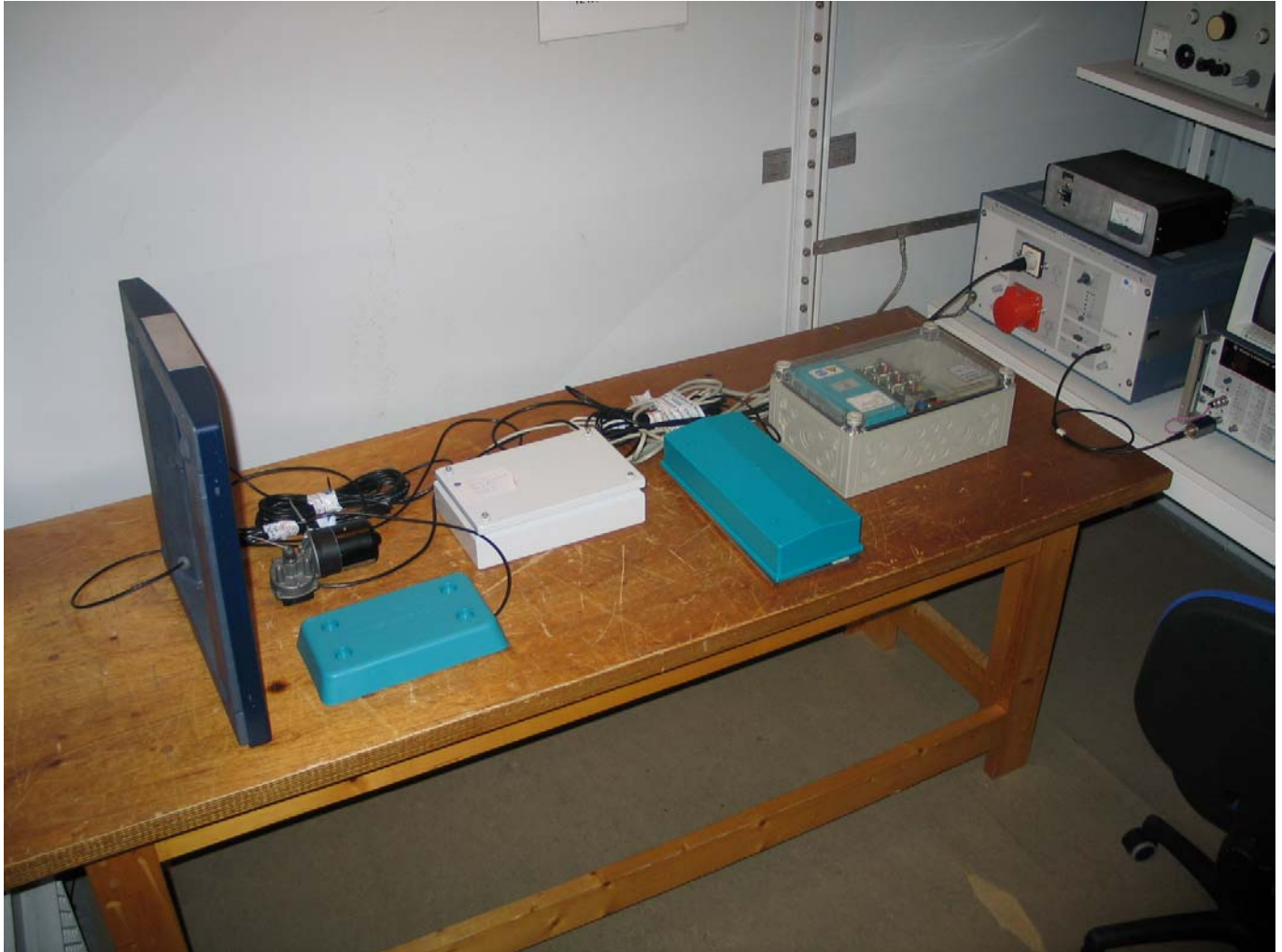
Photo 6: Conducted emission measurement set up
