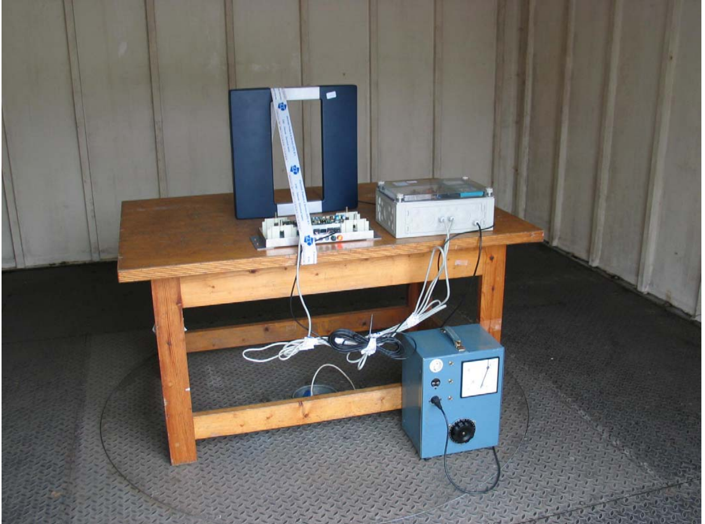
Photo 3: Radiated Emission measurement set up, rear view, with medium V-sense
