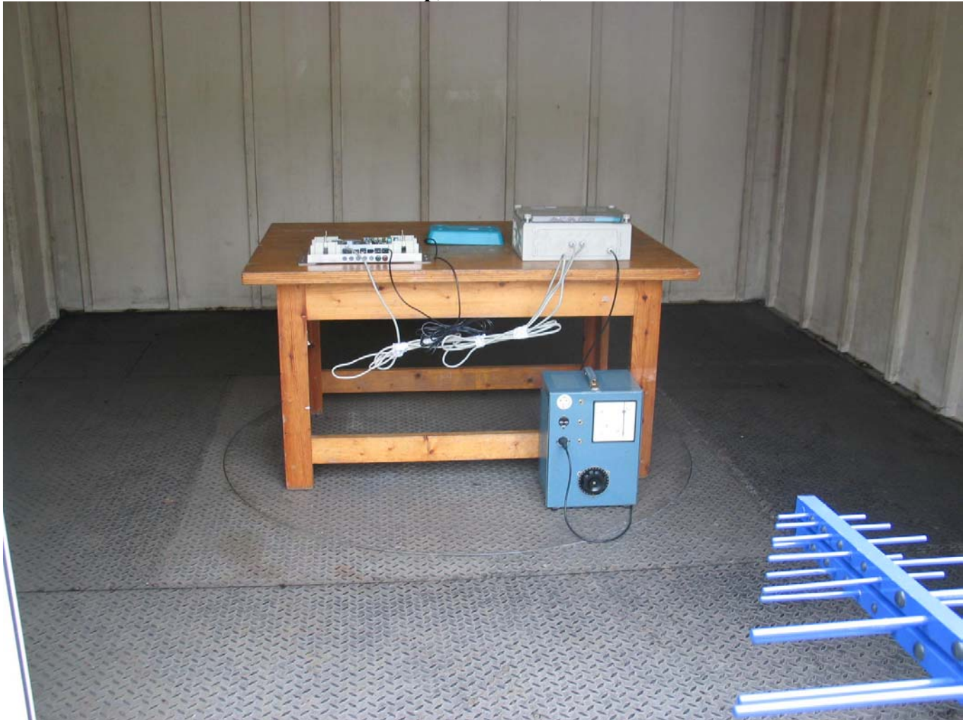
Photo 2: Radiated Emission measurement set up, front view, with small V-sense, rear view
