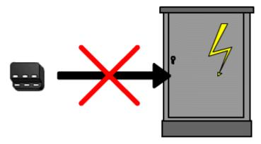
Note: The control unit must never be installed in a metal power cabinet. This would impede wireless communication.
