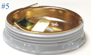
Apply Lube Before “O” Ring
