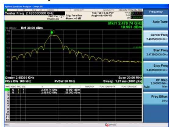
Zigbee, Channel No.: 26
