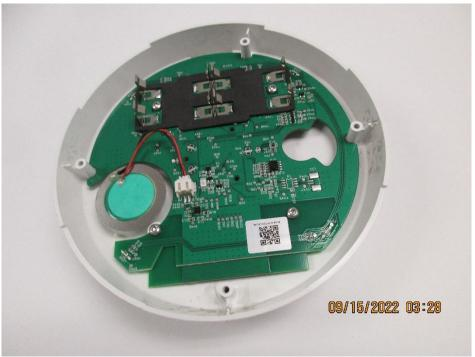
Figure 1 PCB with Battery holder]
