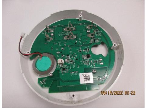
Figure 3 PCB without battery holder
