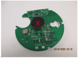
Figure 5 SIXCOMBOV with smoke chamber
