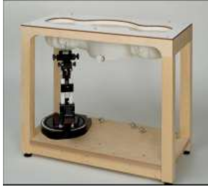
Picture C.8: SAM Twin Phantom
