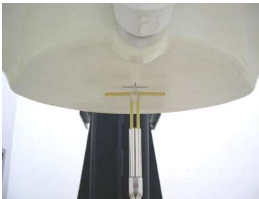
Picture 8.2 Photo of Dipole Setup
