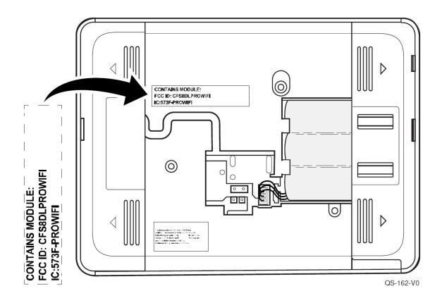
For the GRIP Hybrid, label is to be placed by the installer on the inside door in the location shown:
