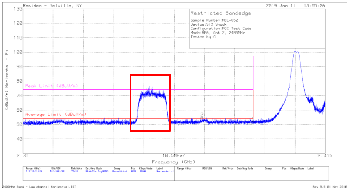
Antenna 2: Low Channel Horizontal – Plot
