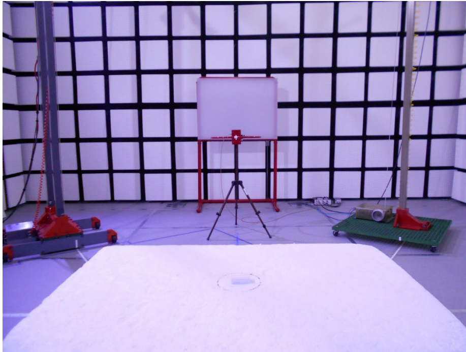
RADIATED BELOW 30MHz FLAT
