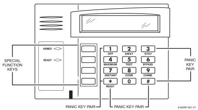
6160RF Keypad/Transceiver (front door removed)
