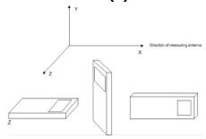
When an emission was found, the table was rotated to produce the maximum signal strength. At this point, the antenna was raised and lowered from 1m to 4m. The antenna was placed in both the horizontal and vertical planes.
