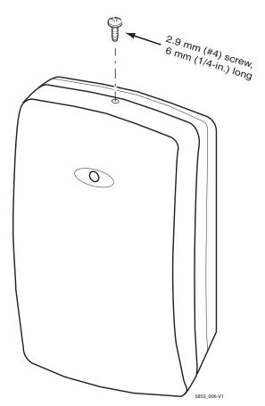
Alternatively, when heavy window coverings are present, the detector can be mounted on the frame of the window.
