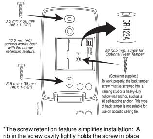
when installing the detector.
