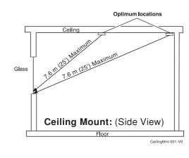
NOTE: If the device is ceiling mounted, the end with the hole (Microphone end) should face the protected glass.
