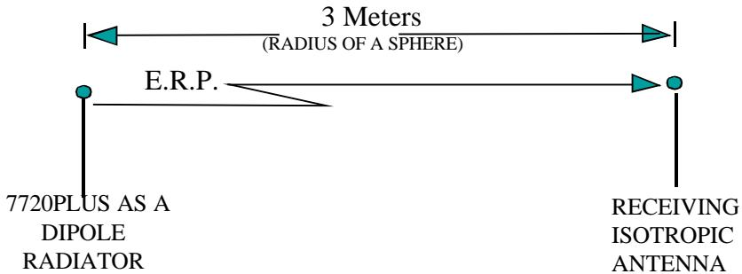
Let the 7720PLUS be a Radiator having the gain of a dipole at the center of a sphere that has a radius of 3 meters (test range distance).
