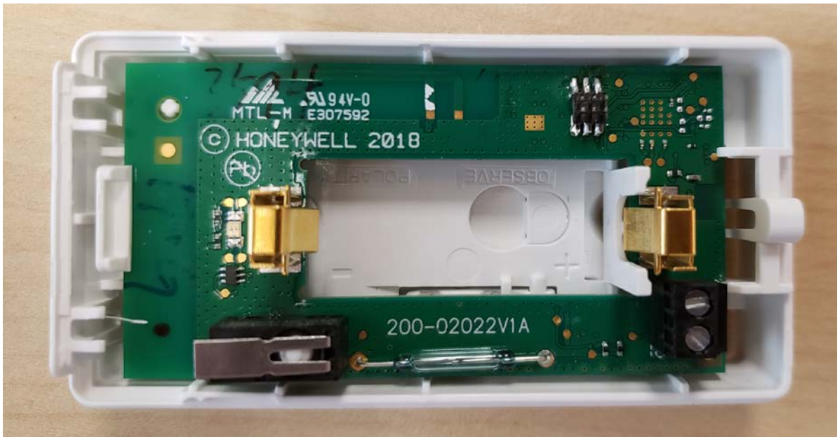
CASE INTERIOR WITH PCB INSTALLED
