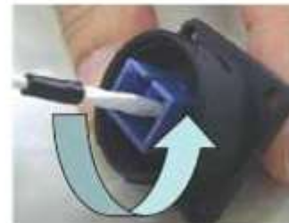
When cleaning stick do not penetrate, rotates several times in a same direction and take care for wary sleeve damage.
