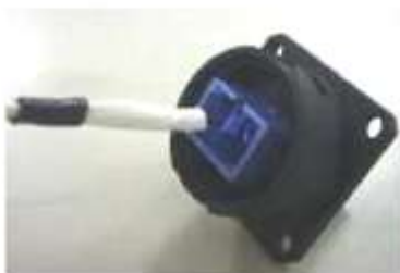
Cleaning stick inserts to the wary sleeve
