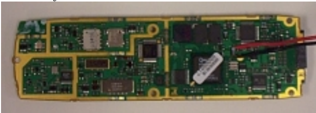
RX Side of the main circuit board
