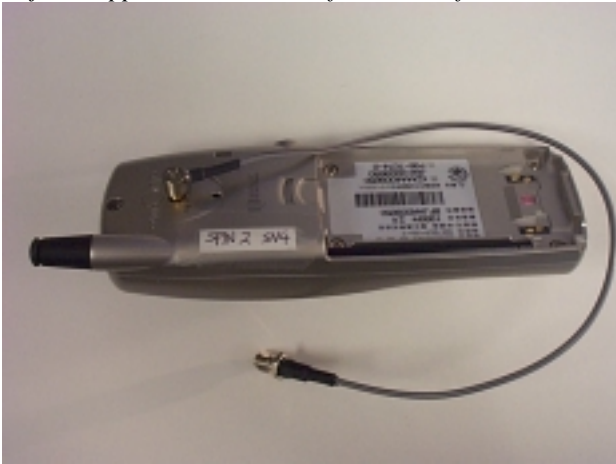
Fujitsu-supplied RF test cable for RF interface
