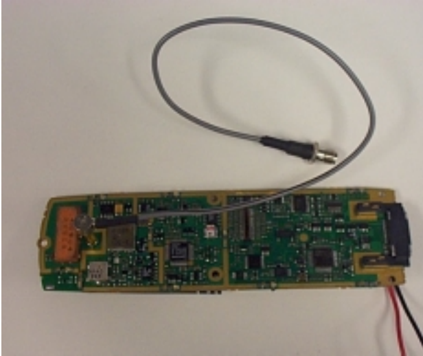
RF access port near antenna interface
