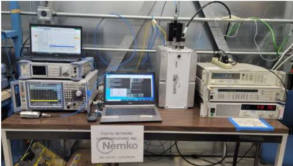
Figure 5 – Test setup (power meter measurements)
