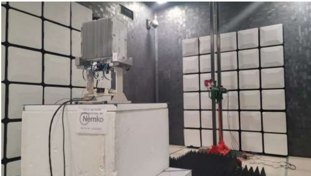
Figure 4 - Radiated emissions above 1 GHz (1 – 7 GHz), rear view.
