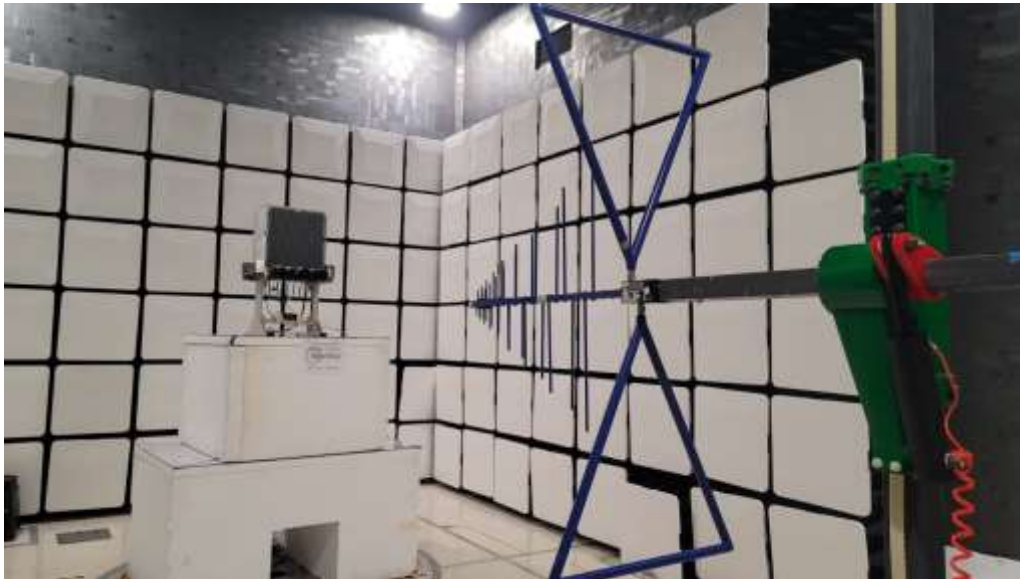
Figure 1 - Radiated emissions below 1 GHz (0.03 – 1 GHz), front view.
