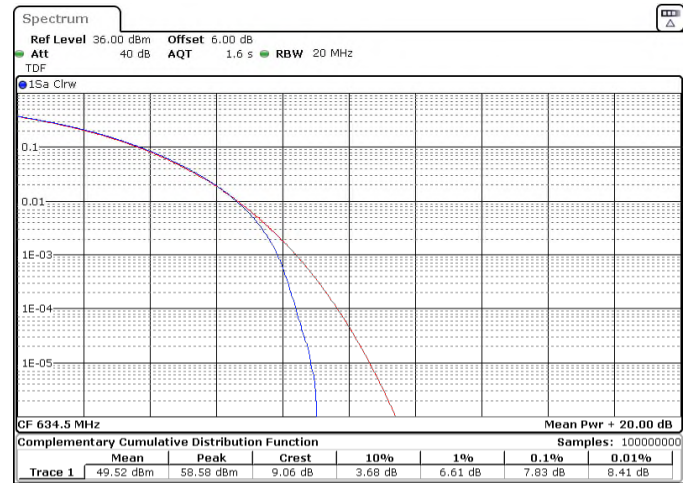
Figure 8.5-4: Peak to average power ratio, 64QAM, Modulation, low channel (15 MHz) and middle channel (15 MHz), respectively.
