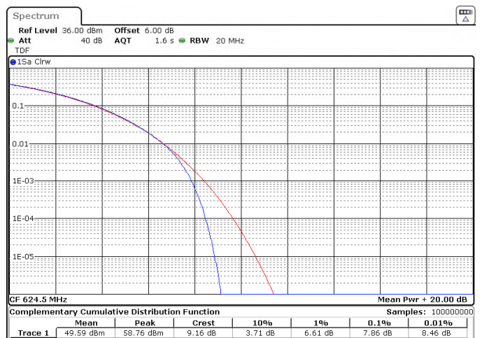
Figure 8.5-5: Peak to average power ratio, 64QAM, Modulation, high channel (15 MHz) and 256QAM, low channel (15 MHz), respectively.
