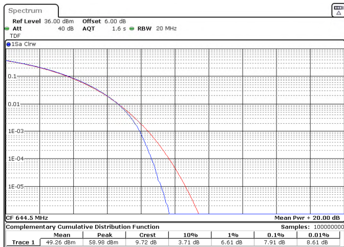
Figure 8.5-5: Peak to average power ratio, 64QAM, Modulation, high channel (15 MHz) and 256QAM, low channel (15 MHz), respectively.
