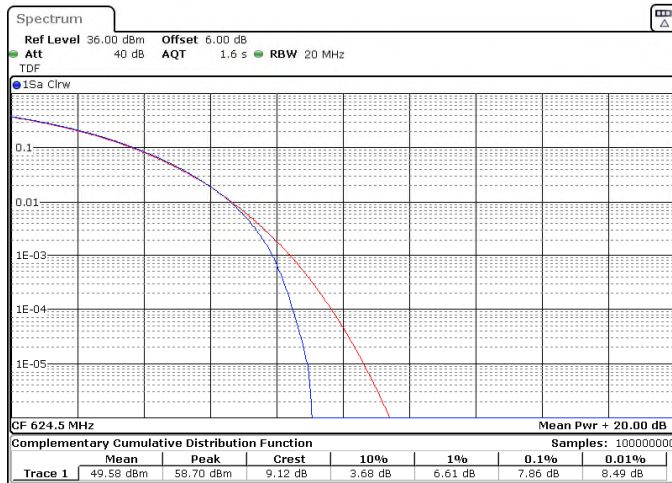
Figure 8.5-4: Peak to average power ratio, 64QAM, Modulation, low channel (15 MHz) and middle channel (15 MHz), respectively.
