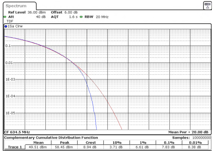
Figure 8.5-1: Peak to average power ratio, QPSK Modulation, low channel (15 MHz) and middle channel (15 MHz), respectively.
