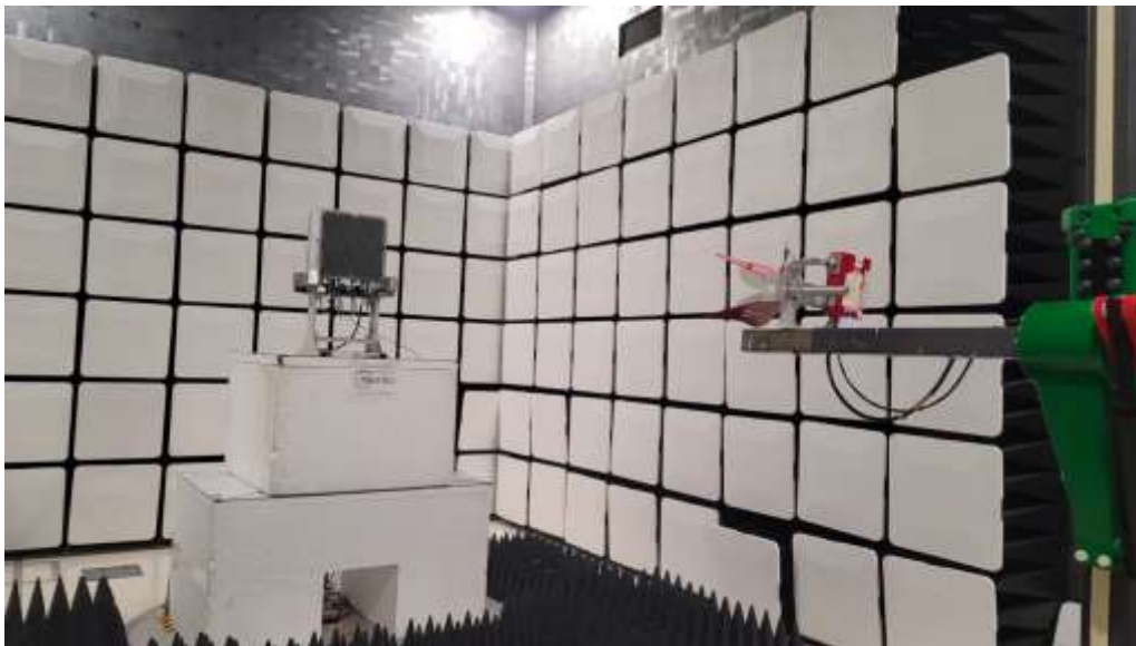
Figure 3 - Radiated emissions above 1 GHz (1 – 18 GHz), front view.
