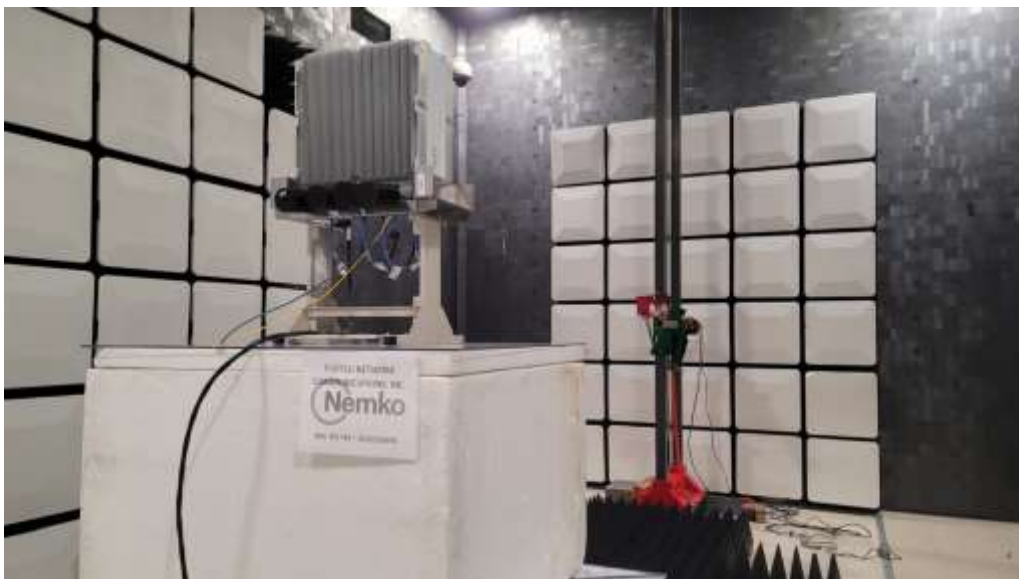
Figure 4 - Radiated emissions above 1 GHz (1 – 18 GHz), rear view.
