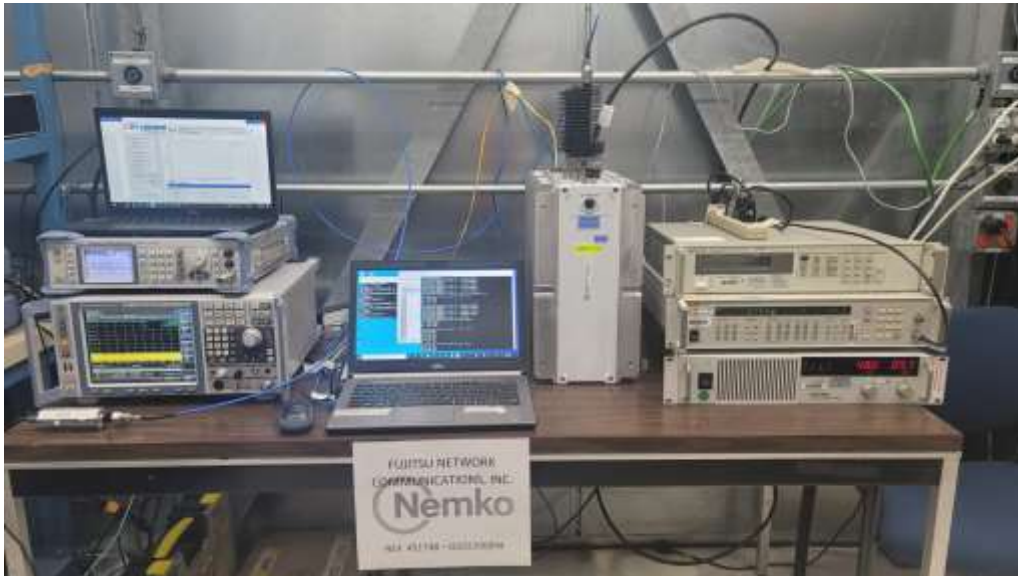
Figure 7 – Test setup (power meter measurements)
