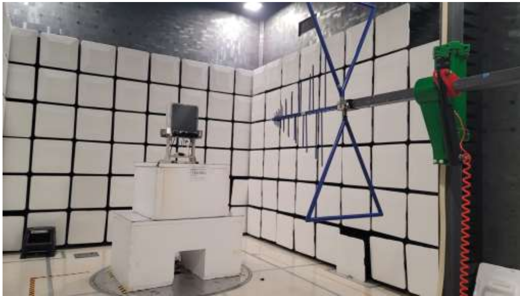
Figure 1 - Radiated emissions below 1 GHz (0.03 – 1 GHz), front view.
