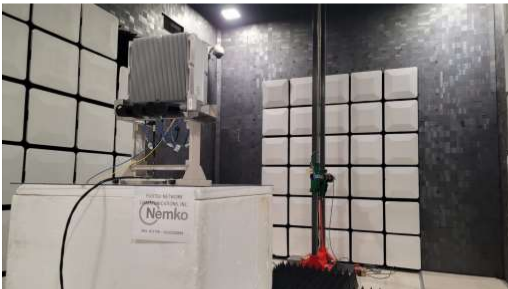
Figure 6 - Radiated emissions above 1 GHz (18 – 26 GHz), rear view.
