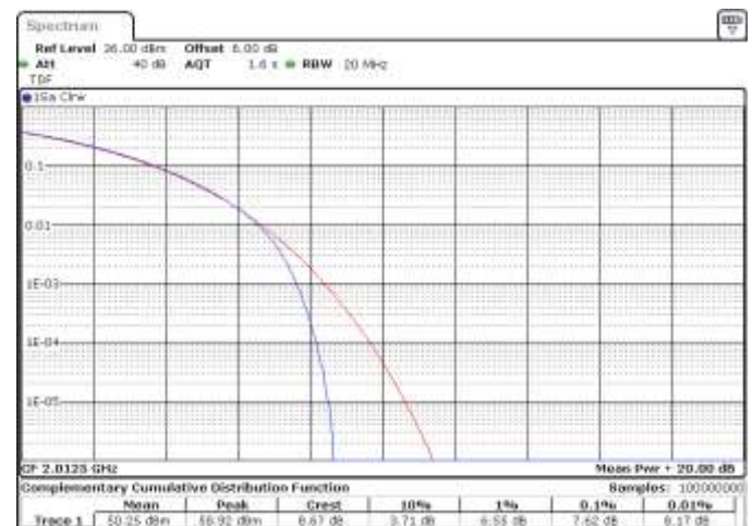
Figure 8.5-7: Peak to average power ratio, QPSK Modulation, low and high channel (15 MHz), respectively, band n70.
