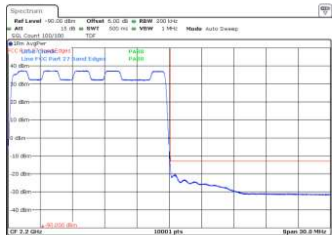
Figure 8.6-12: Conducted emission test, 16QAM Modulation, band edge: low and high channels, respectively (15 MHz), band n66.
