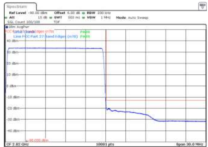
Figure 8.6-28: Conducted emission test, QPSK Modulation, band edge: low and high channels, respectively (15 MHz), band n70.
