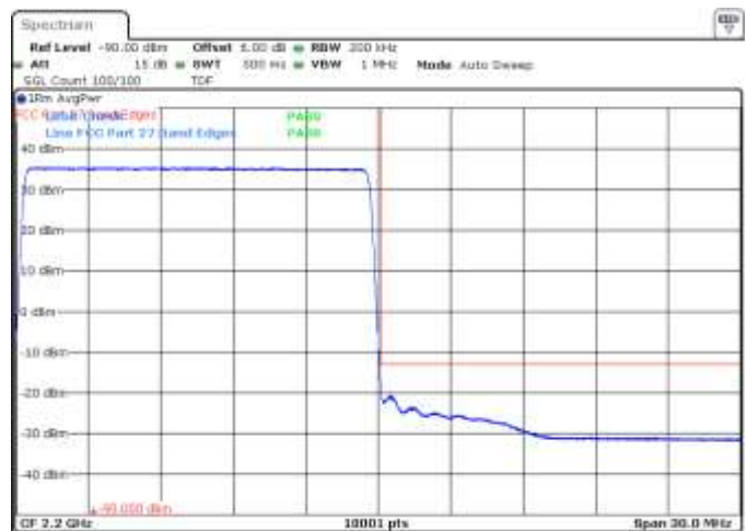
Figure 8.6-24: Conducted emission test, 256QAM Modulation, band edge: low and high channels, respectively (15 MHz), band n66.
