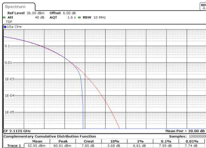
Figure 8.5-1: Peak to average power ratio, QPSK Modulation, low and middle channel (5 MHz), respectively, band n66.
