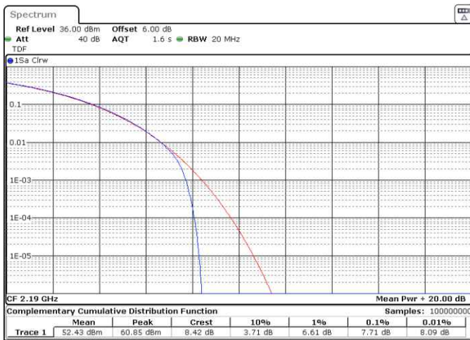
Figure 8.5-5: Peak to average power ratio, QPSK Modulation, high channel (10 MHz), band n66 and 2007.5 channel (25 MHz), band n70, respectively.
