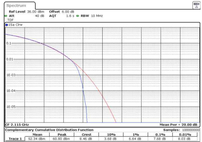
Figure 8.5-2: Peak to average power ratio, QPSK Modulation, high channel (5 MHz) and low channel (10 MHz), respectively, band n66.
