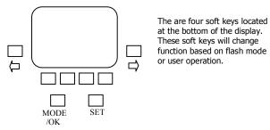
The **Mode** button allows you to change the mode of the Trio. Pushing it will bring up the mode change menu.
