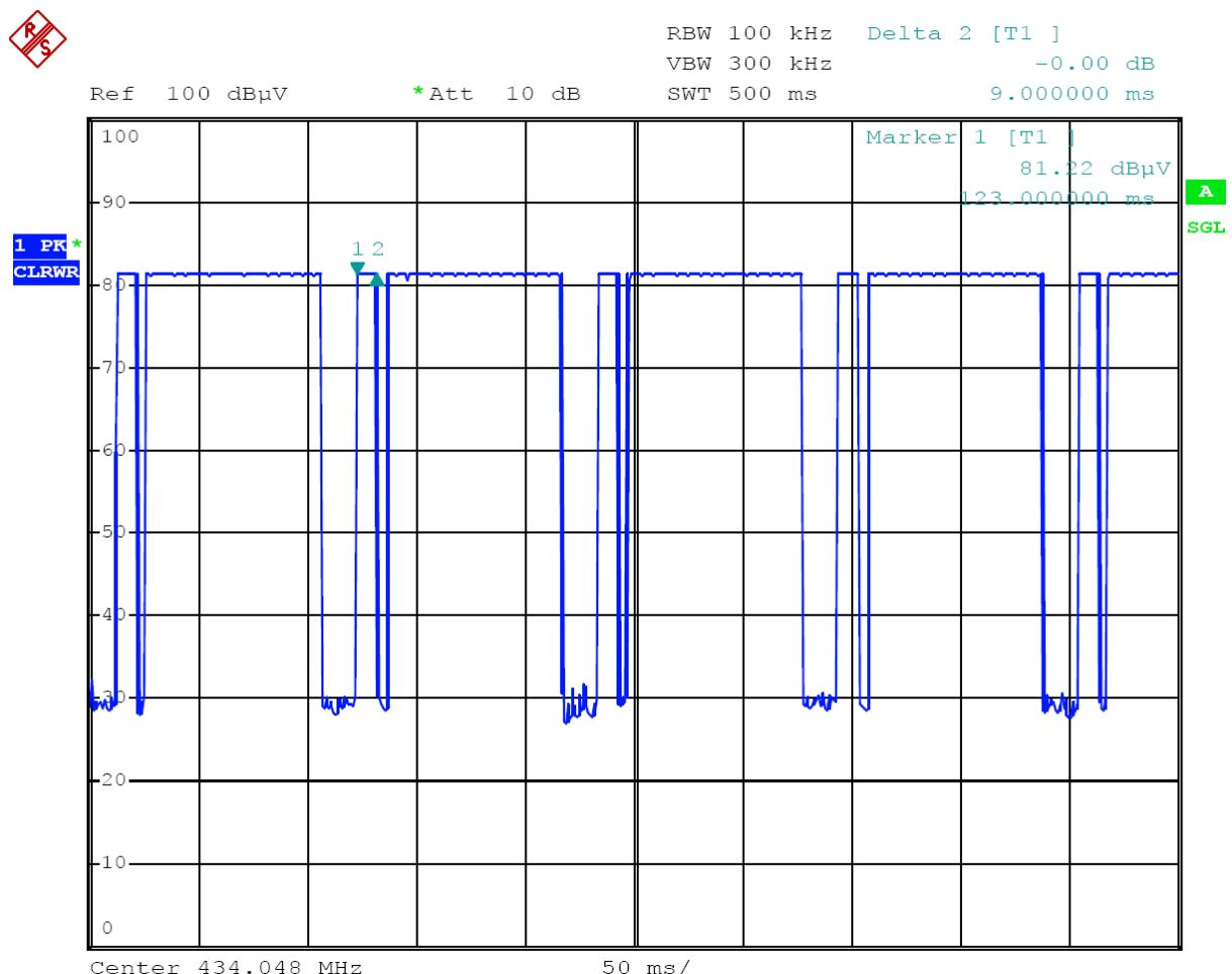
The graph shows the duration of short 'on' signal. From marker 1 to marker 2, duration is 9ms.
