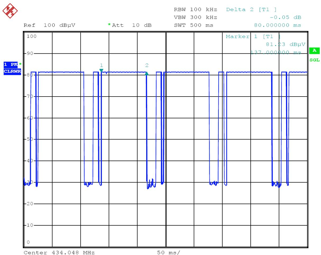
The graph shows the duration of long 'on' signal. From marker 1 to marker 2, duration is 80ms.
