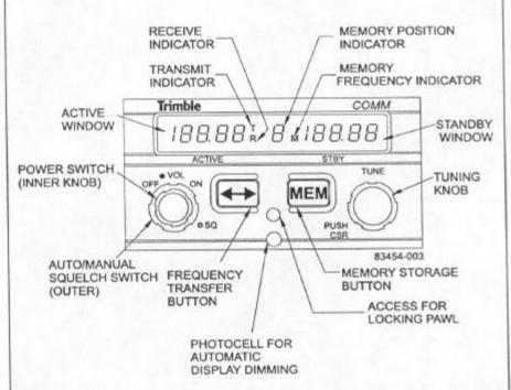
The active frequency is displayed on the left side of the display window and the standby frequency is displayed on the right side. The TC100 displays a "T" to the right of the active frequency during transmit and displays an "R" when the transceiver is receiving. When the TC100 is in memory transfer mode, it displays an "M" to the left of the standby frequency. The memory position number is displayed between the active and standby frequencies.
