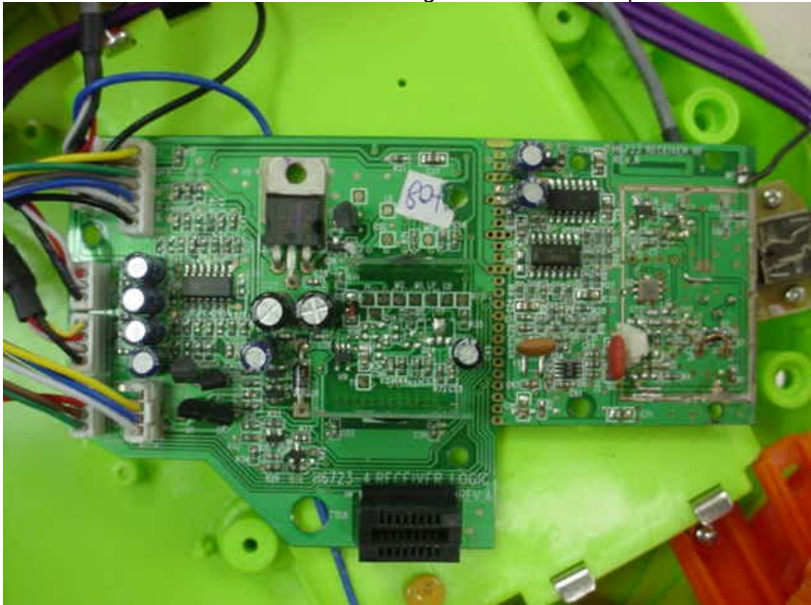
Fisher-Price H6723 Receiver with Shielding Can removed – Top View
