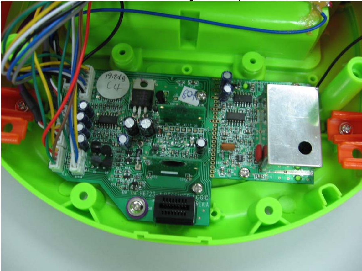
Fisher-Price H6723 Receiver with Shielding Can removed – Top View
