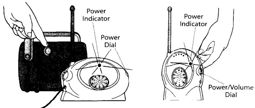
Place transmitter in room in which you intend to use it. Rotate transmitter power dial to turn power on. Power indicator lights. Turn on a radio.
