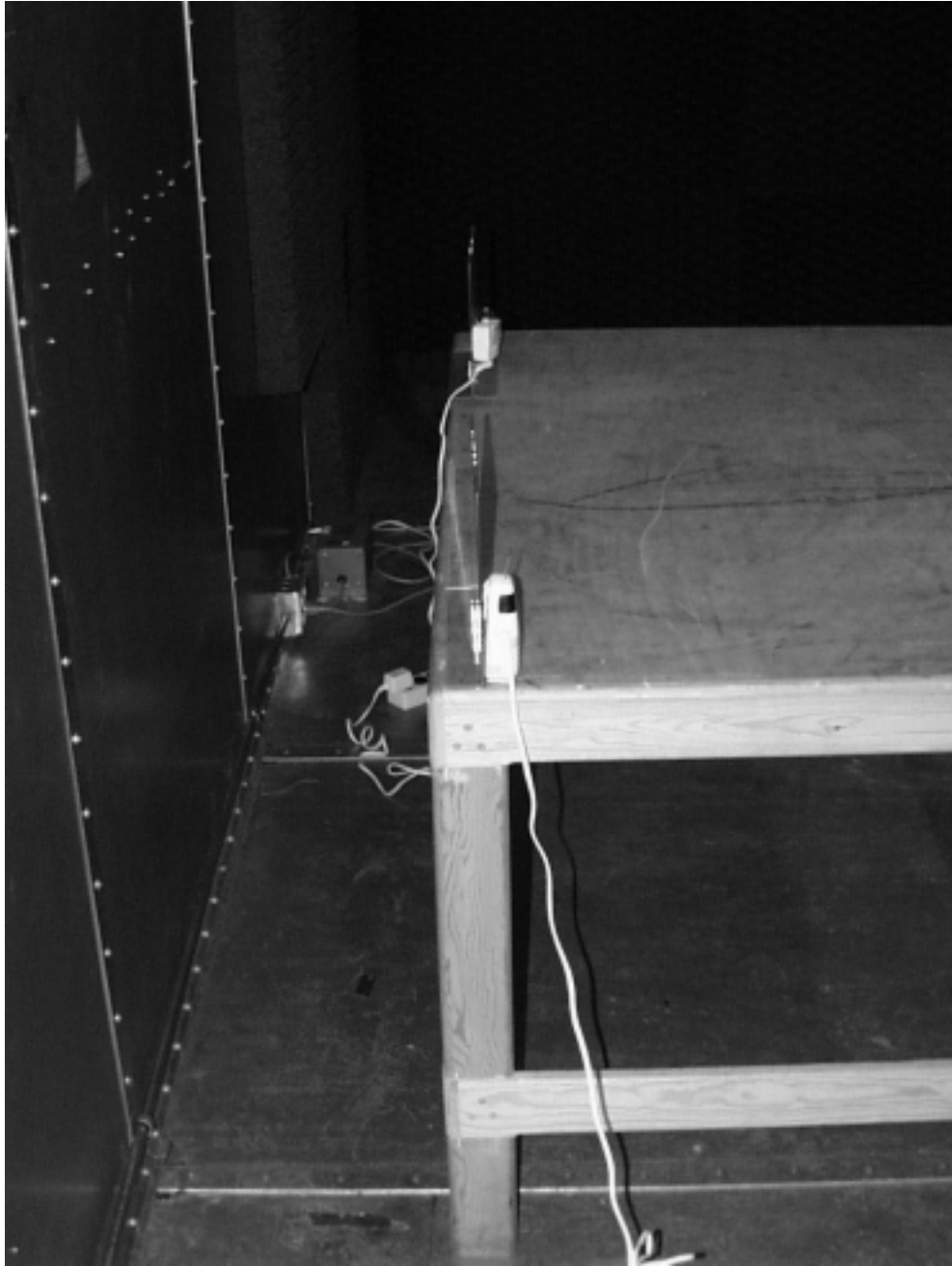
Conducted Emissions, Side View
