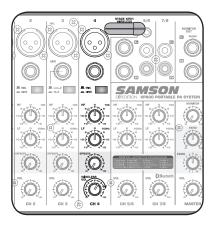
Raise the MASTER LEVEL control and speak or sing into the mic at a normal performance level while raising the Channel 4 LEVEL control until the desired level is reached.
