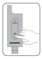
If the handheld transmitter and receiver have not been previously paired, press and hold the button on the RXD1 receiver for >5 seconds, until it begins to flash.
