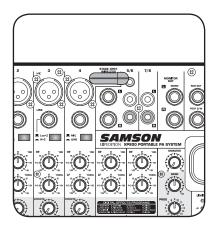
Turn the channel 4 LEVEL knob on the XP800 completely counterclockwise to 0, then turn the POWER siwtch on the XP800 to the ON position.
