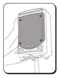
6. Using one of the included speaker cables, connect the mixer's LEFT SPEAKER OUT to the left speaker's input connector. Next, use the second included speaker cable to connect the RIGHT SPEAKER OUT to the right speaker's input connector.
