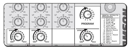
The XP300 input channels feature a 2-band equalizer allowing you to adjust the tonal characteristic of the signal. You can independently adjust the bass and treble frequencies on each channel. The channel's frequency response is flat when the knobs are in the 12 o'clock position.
