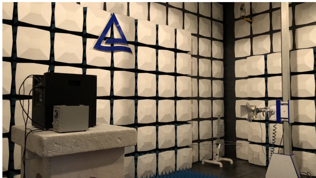
Photograph 2: Set-up for Radiated Spurious Emission, Above 1GHz
