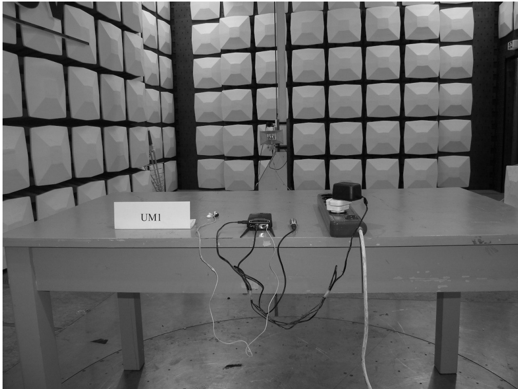
Photograph 3: Set-up for Radiation Measurement above 1GHz
