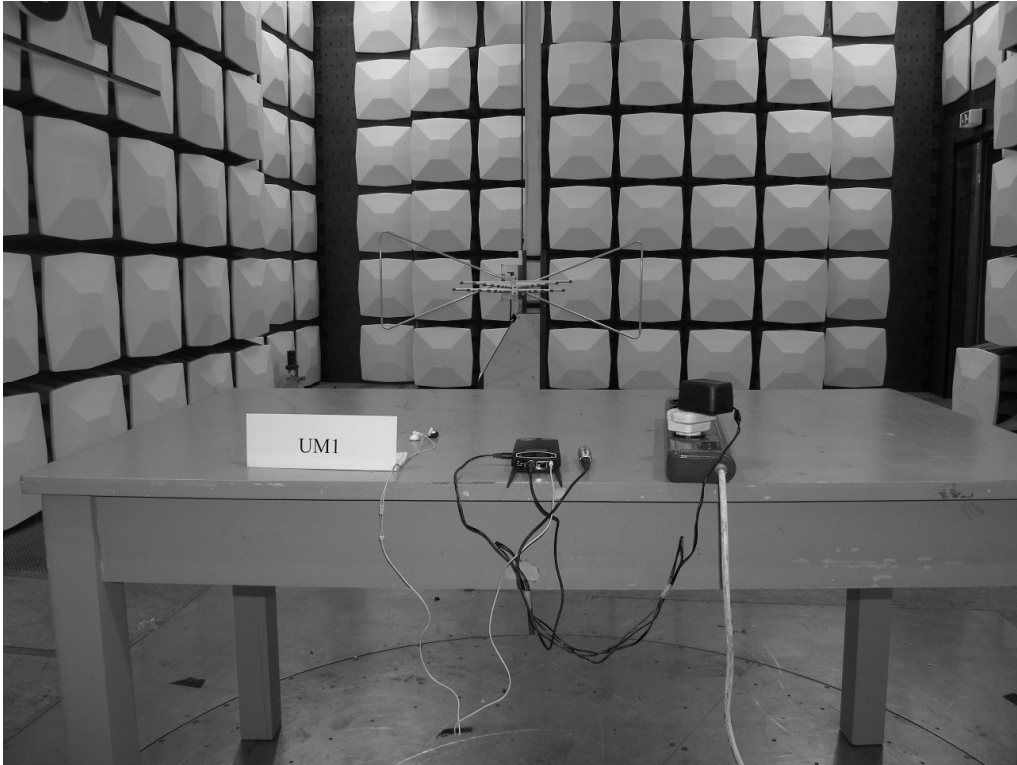
Photograph 2: Set-up for Radiation Measurement below 1GHz
