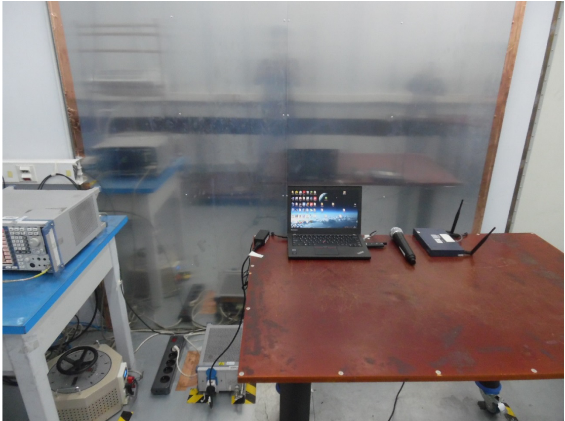
Photograph 1: Set-up for Conducted Emission
