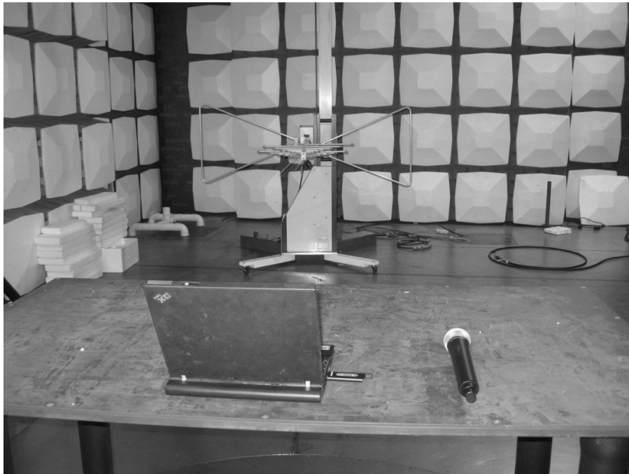
Photograph 2: Set-up for Radiated Emission (30MHz-1GHz)
