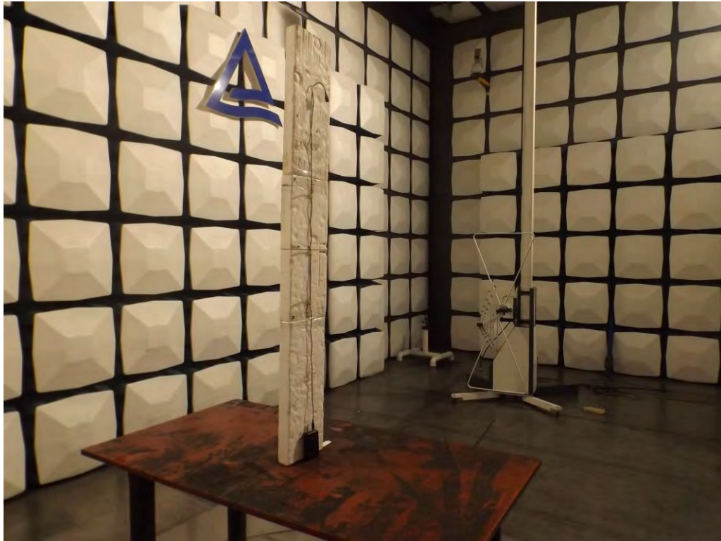
Photograph 1: Set-up for Radiation Measurement below 1GHz
