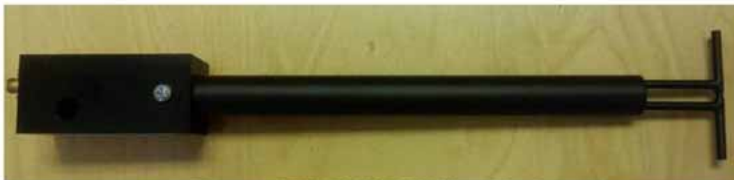
Figure 1 – MVG COMOSAR Validation Dipole
