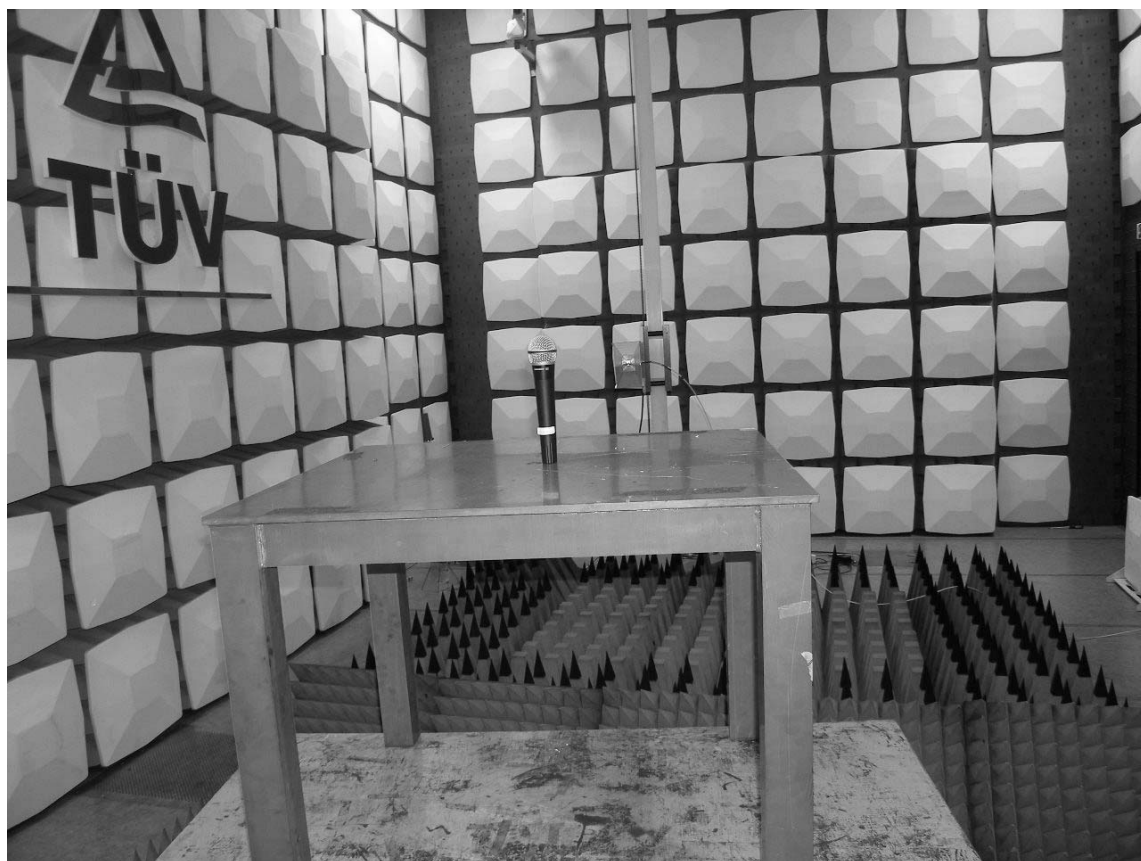
Photograph 2: Set-up for Radiation Measurement above 1GHz
