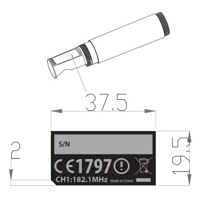
2. SERIES NUMBER AND FREQUENCY LABEL STUCK ON THE BATTERY COMPARTMENT OUTER HOUSING
