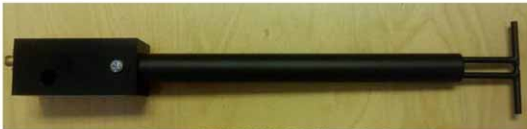
Figure 1 – MVG COMOSAR Validation Dipole
