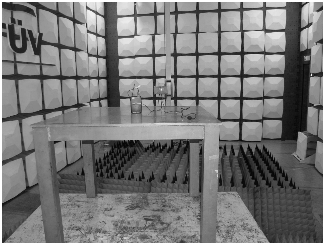
Photograph 2: Set-up for Radiation Measurement above 1GHz
