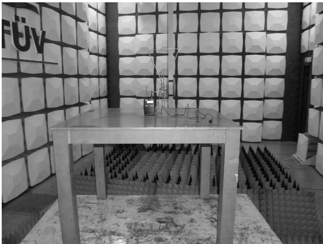
Photograph 1: Set-up for Radiation Measurement Below 1GHz
