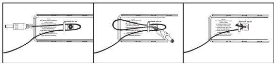
Using the strain relief: Gather up a loop of wire and pass it through the strain relief, then pass the adapter plug through the loop in order to create a knot.
