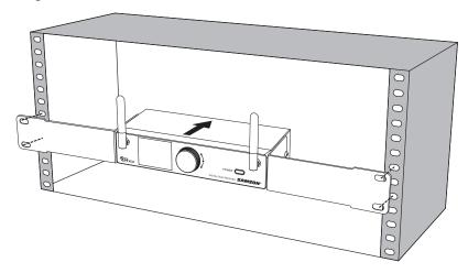
Mount the receiver into the rack using the appropriate size rack screws (not included). To ensure equal tension and balance when installing the receiver, you should secure screws in a crisscross pattern of opposite corners: top left -> bottom right -> top right -> bottom left.
