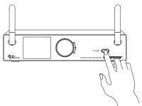
**6.** Turn on the power to the CHXD2 transmitter by pressing and holding the power/mute button; the indicator LED will light YELLOW, then changes to GREEN when the power/mute button is released (if properly paired).
