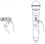
7. Turn on your connected amplifier or mixer, but keep the volume all the way down. Speak or sing into the microphone at normal performance level. Slowly raise the volume of your amplifier or mixer until the desired volume level is reached.
