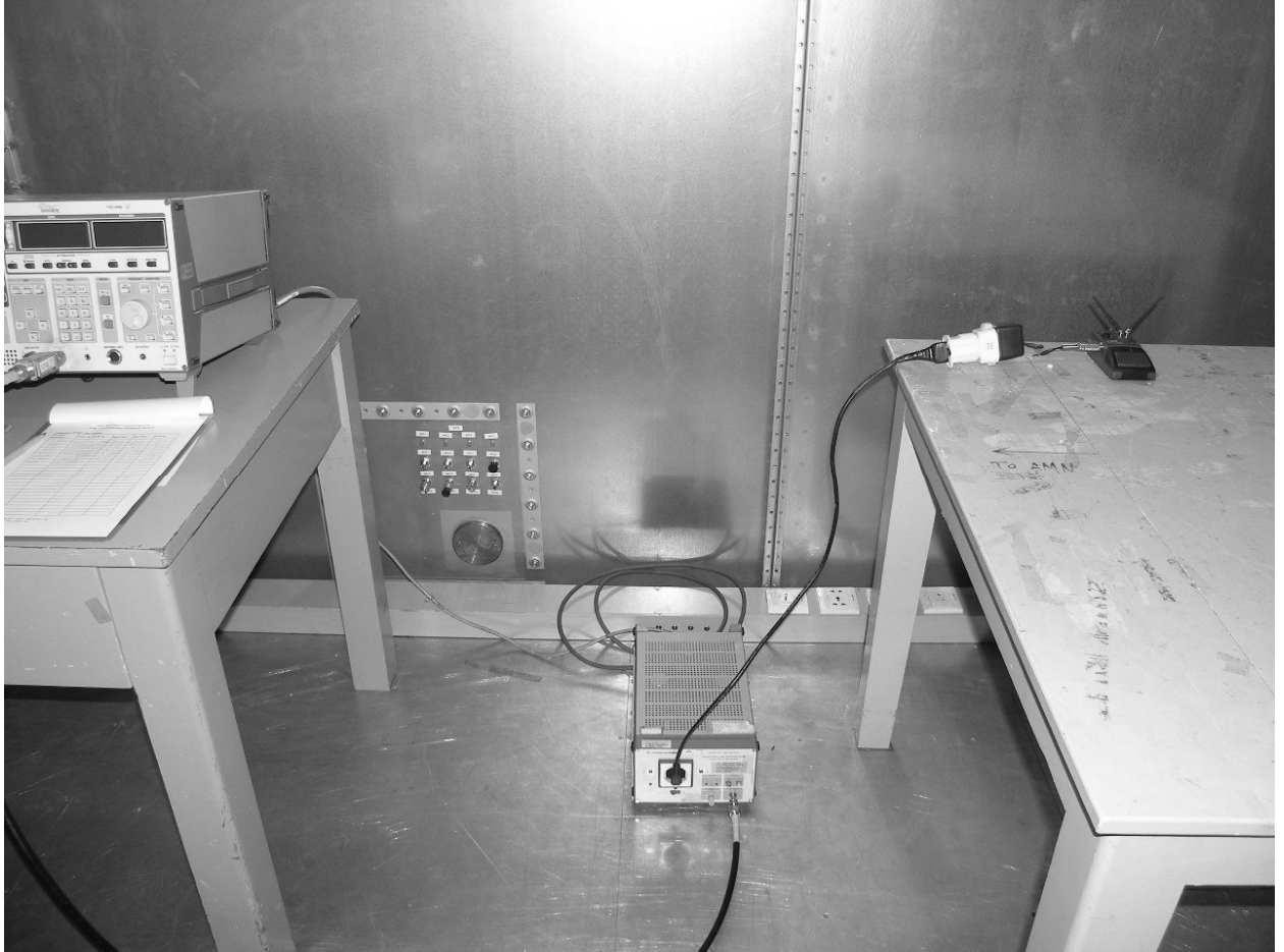
Photograph 1: Set up for Conducted Emission on AC Mains
