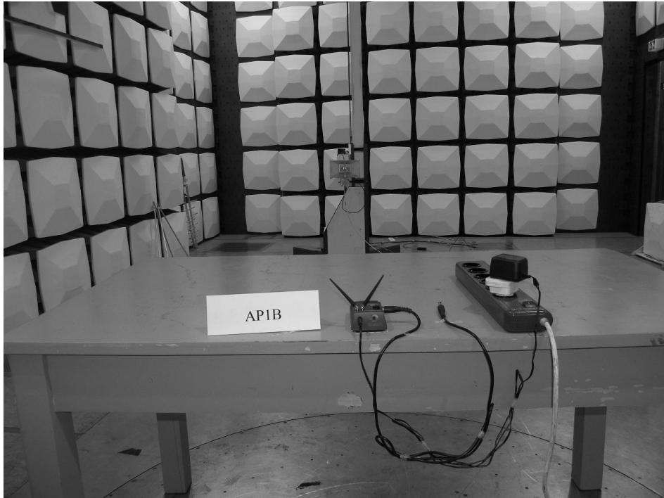
Photograph 3: Set-up for Radiation Measurement above 1GHz
