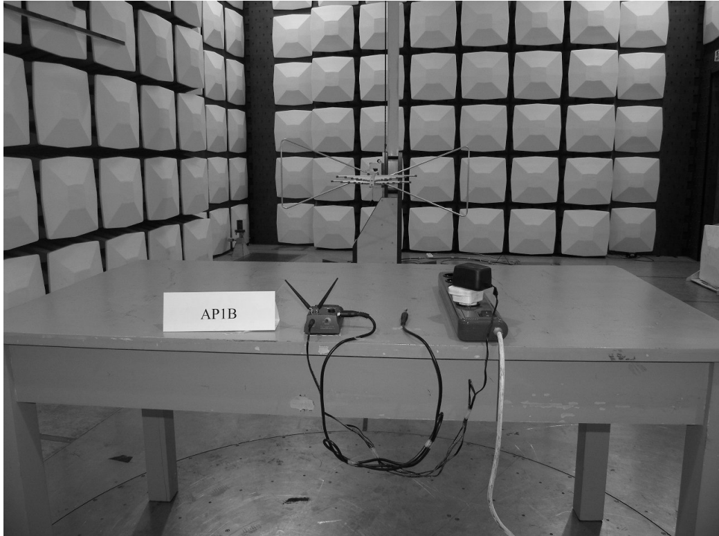
Photograph 2: Set-up for Radiation Measurement below 1GHz
