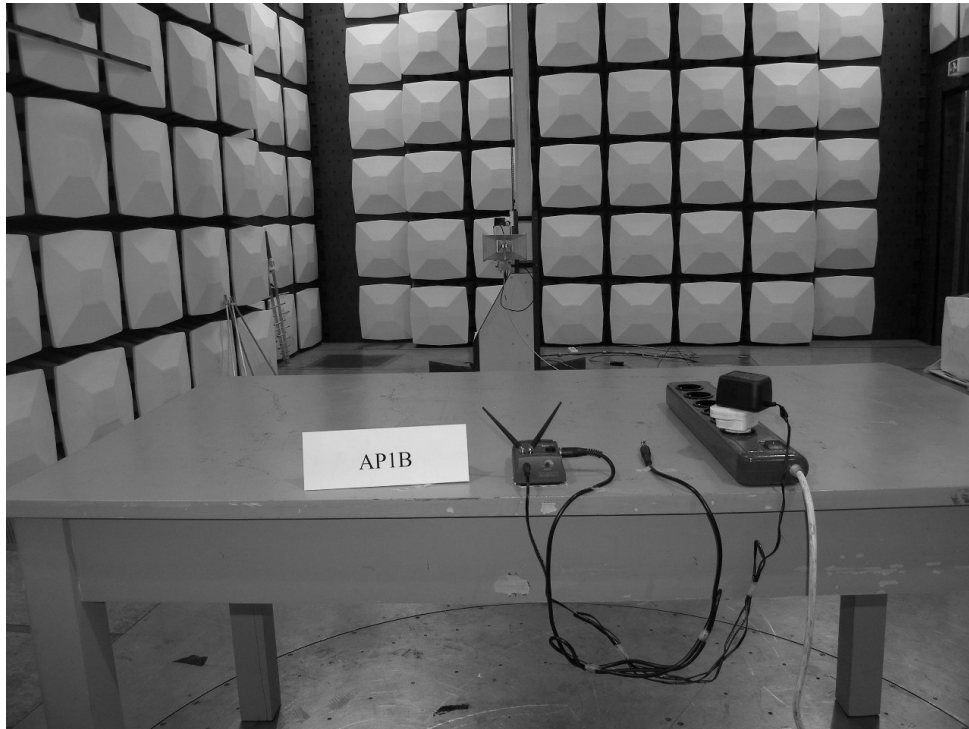
Photograph 3: Set-up for Radiation Measurement above 1GHz
